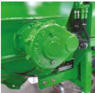
Gearbox drive for agitator
